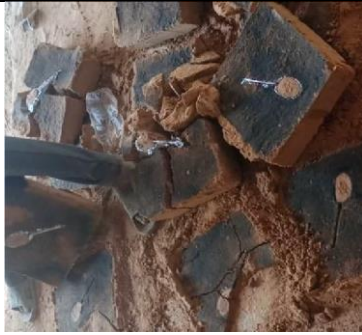
7. Breaking the mold to remove Cast
