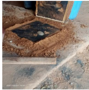
4. After ramming the Mold 5. Removing the Pattern 6. Pouring the hot metal
