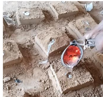
4. After ramming the Mold 5. Removing the Pattern 6. Pouring the hot metal
