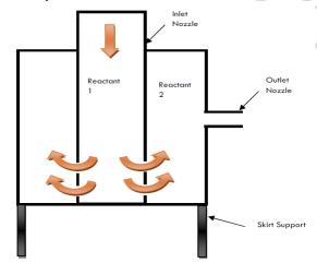
Fig. Block diagram of Reactant Column
