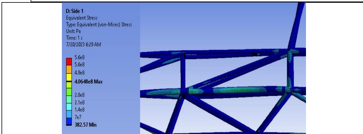
Figure C.3.A: FEA of side impact 1 – equivalent stress
