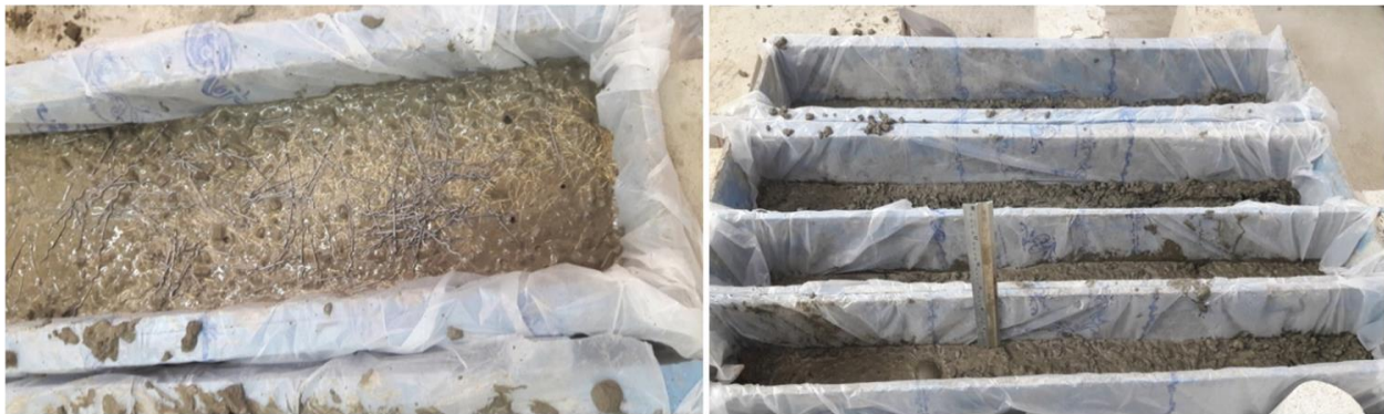
Fig. 2: Layered casting of concrete using steel-brass hybrids.
