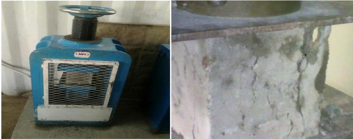
Figure 1:- Concrete Cube Specimens before Failure Figure 2:- Concrete Cube specimen after Failure
