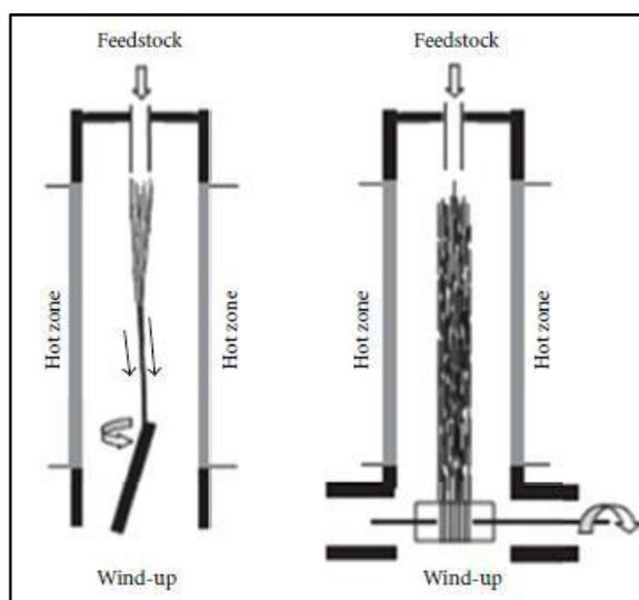
Fig: Schematic of the direct spinning process
