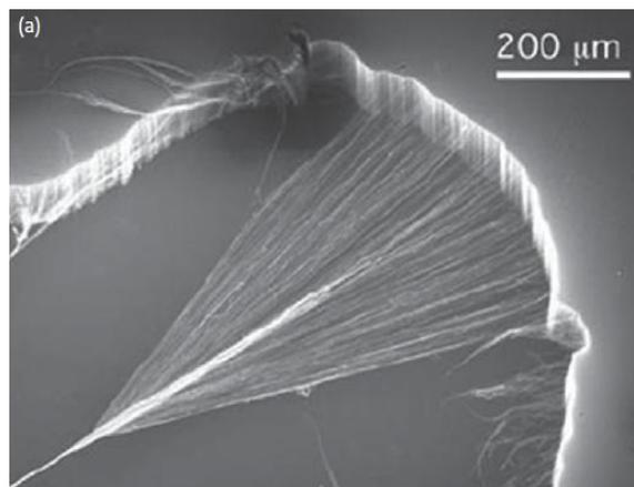
Fig. 4 Scanning electron microscopy images of a carbon nanotube yarn twisted during solid-state spinning. (Reproduced from Zhang et al[20])
