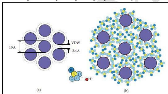
Fig: A model illustrating the swelling of SWNT ropes in sulfuric acid. (a) A cartoon of SWNTs in van der Waals contact within a neat fiber. (b) The same SWNT fiber after reexposure to sulfuric acid [16]
