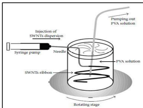
Fig: Schematic of the rotating bath used for coagulating surfactant-dispersed SWNTs into a fiber
