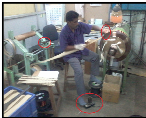
Fig.2: Semi-Automatic Transformer winding machine.
