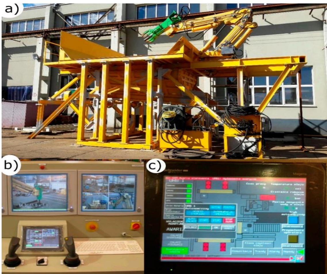
Figure 7. Station for testing; (a) autonomous equipment; (b) operator's panel; (c) GUI (Graphical User Interface) view
