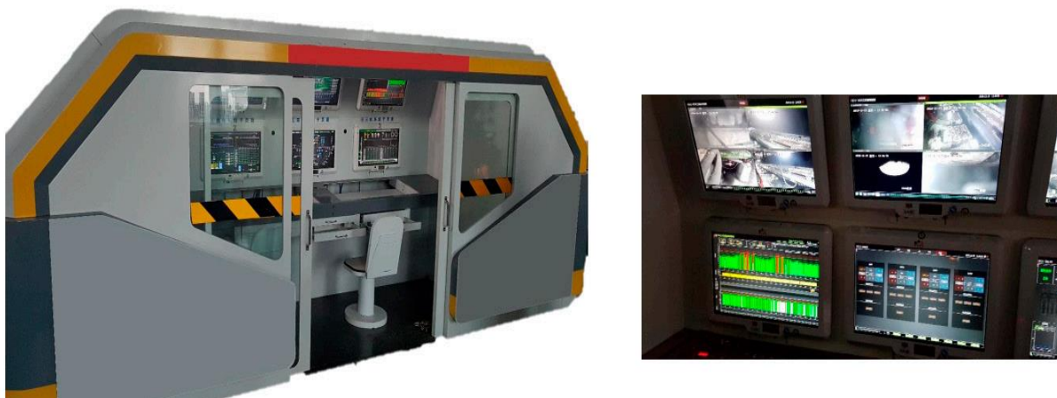
Figure 2. Cabin for monitoring the automatic operation of the MIKRUS system from the surface
