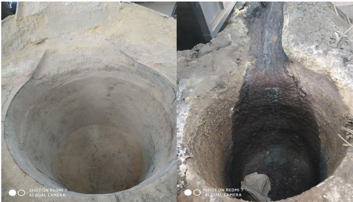
2 – picture. The condition of the inner layer of the induction furnace after melting the wear – resistant white iron
