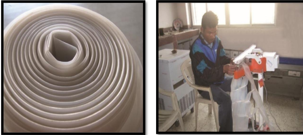
Figure.1: Peddle machine preparation of plastic cell formwork
