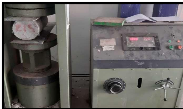
Fig.7. Split tensile strength test
