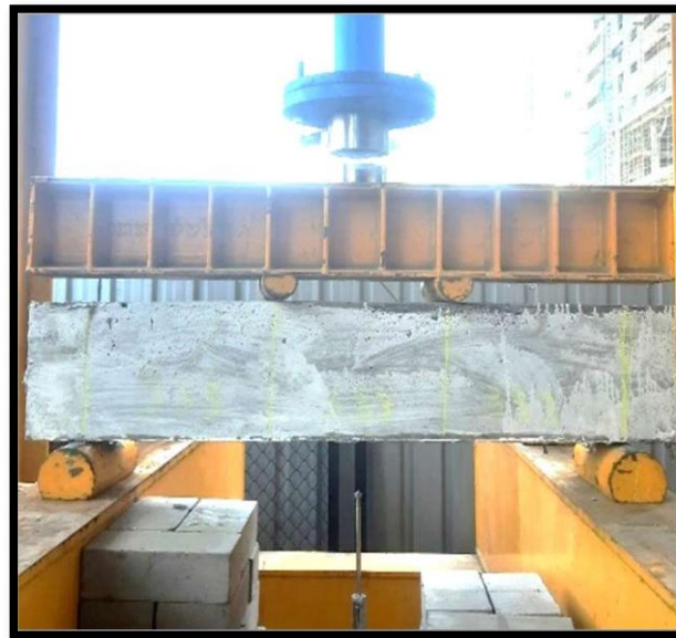
Fig. 4. Two-point load test setup
