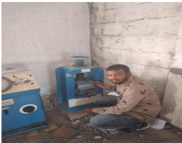
Figure 3 - Compressive strength testing on CTM
