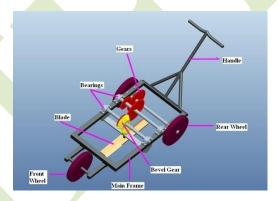
**Figure 1:** 3D model of the lawn mower
