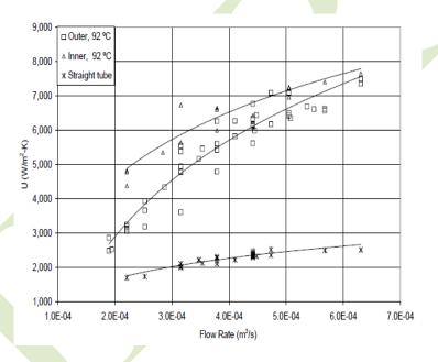
Fig.12 U in helical heat exchangers of different coil diameters as a function of flow rate
