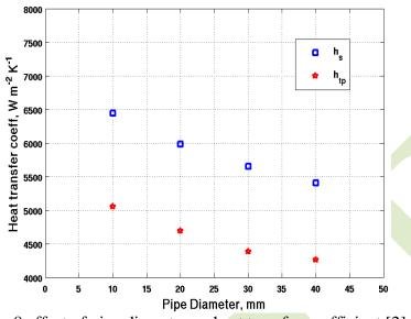
Fig.8 effect of pipe diameter on heat transfer coefficient [2]
