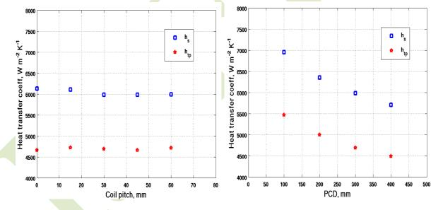
Fig.6 effect of coil pitch on heat transfer Coefficient [2]
