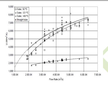
Fig.11 U in straight and helical heat exchangers function of NRe
