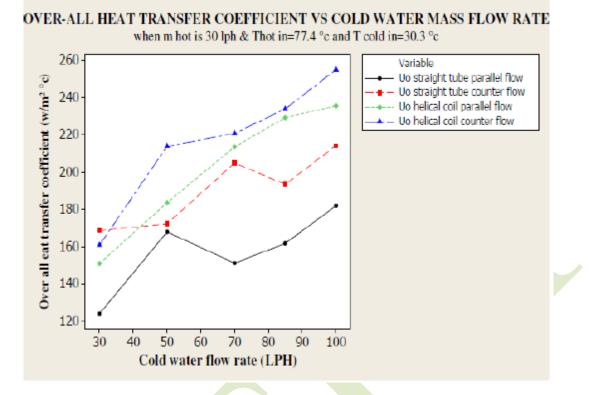
ig.9 variation of overall heat transfer coefficient when mass flow rate inside the tube is 30 LPH.[7]
