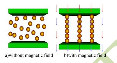
Fig.1. Working principle of MR fluid technology
