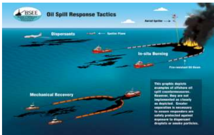
Figure 3: Oil spill response tactics (BSEE)
