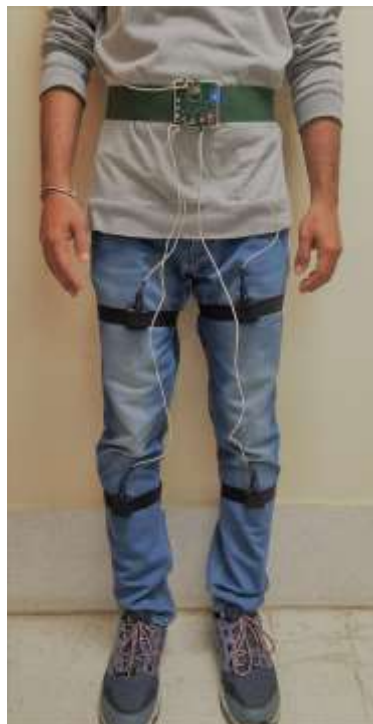
Figure 13: Subject with wearable gait motion analyzer system
