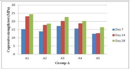
Fig.6 the results of compressive strength test in group A with w/c of 0.5
