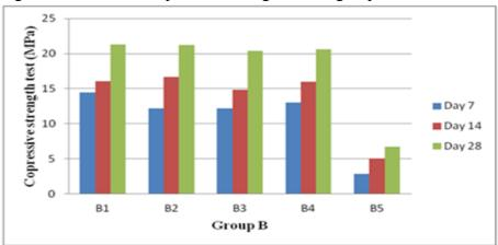
Fig. 7: the results of compressive strength test in group B with w/c 0.55
