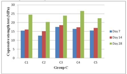
Fig. 8: the results of compressive strength test in group C with W/C of 0.6
