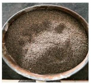
Fig.1 a. Recycled fine aggregate
