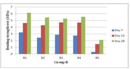
Fig4: bending strength test in group B with w/c of 0.55
