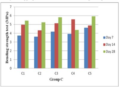
Fig 5: bending strength test in group C with W/C of 0.6
