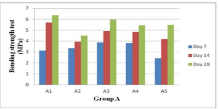
Fig 3: bending strength results in group A with W/C of 0.5
