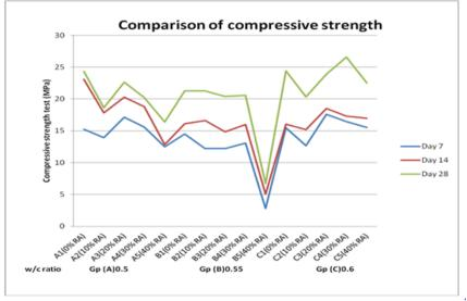
Figure .9: comparing the compressive strength at 7 days, 14 days and 28 days
