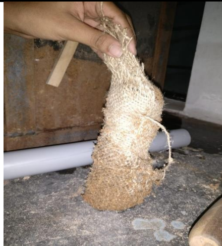
Figure 2: Geosynthetic stone column
