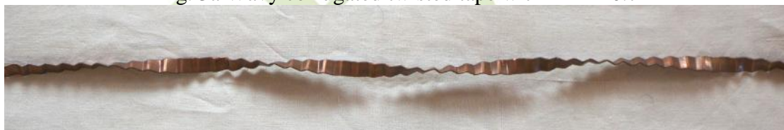
Fig. 3b Wavy corrugated twisted tape with TR – 8.5
