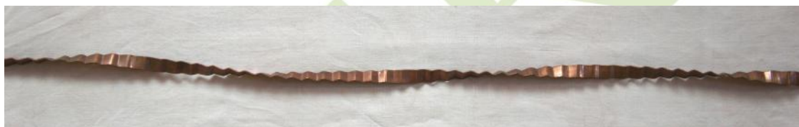
Fig. 3a Wavy corrugated twisted tape with TR – 10.7
