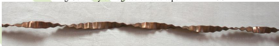
Fig. 3c Wavy corrugated twisted tape with TR – 7.1
