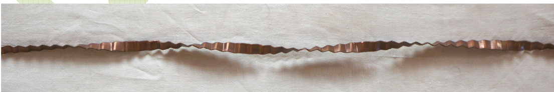
Fig. 5 Wavy corrugated twisted tape with TR – 8.5
