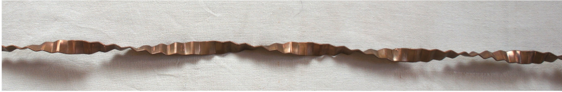
Fig. 6 Wavy corrugated twisted tape with TR – 7.1
