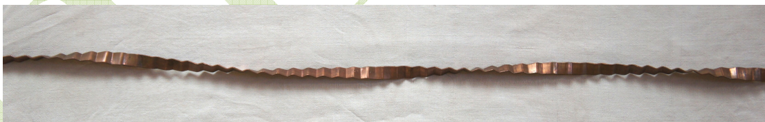
Fig. 4 Wavy corrugated twisted tape with TR – 10.7
