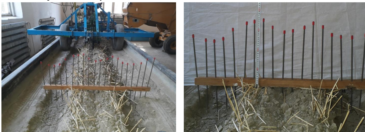
Figure 6. Post-processing of the ripper profile and its detection process
