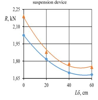
Figure 2. The change in the tensile strength (R) of the housings depending on the longitudinal distance (L6) between them is shown in Figures 1 and 2, respectively, with operating speeds of 6 and 9 km / h.
