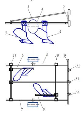
Figure 1. Design scheme of laboratory-field device: 1 - frame; 2 - hanging device; 3 - left and right bodies; 4 - base wheel; 5, 6, 7 and 8 - longitudinal beams; 9, 10, 11 - transverse beams; 12, 13 and 14 - brackets of the
