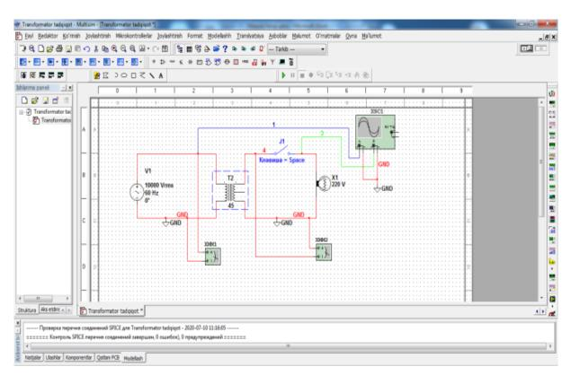
Figure 1. Placement of the research device diagram and measuring control devices in the Multisim program workspace.
