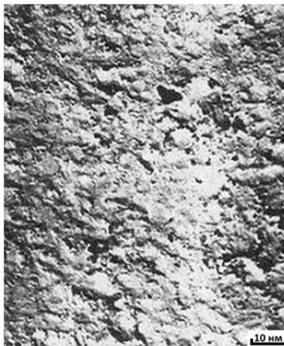
**Fig. 1 SEM of  $\text{CoSiO}/\text{CoSi}_2$  film surface image (100).**
