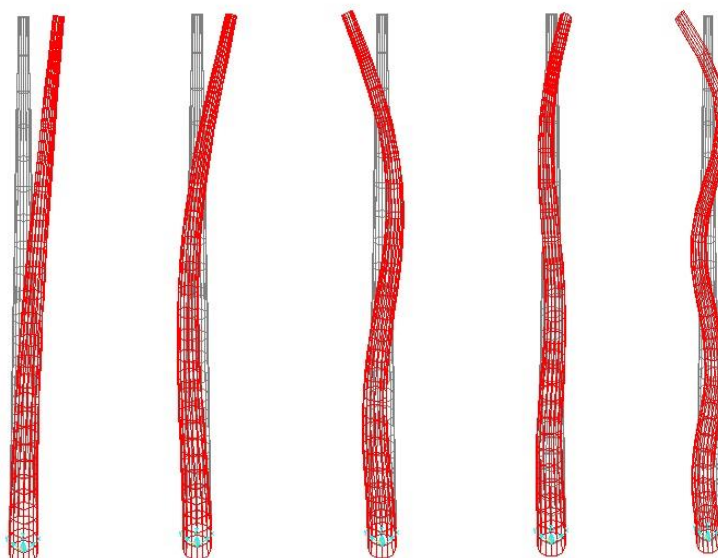
Figure 5. Mode Shapes of Concrete Chimney with CFRP
