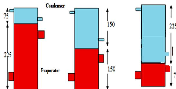
Figure 2: Section ratio of heat pipe heat exchanger 1:3, 1:1 and 3:1
