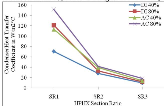
Figure 11: Effect of section ratio and filling ratio of different working fluids on condenser heat transfer coefficient
