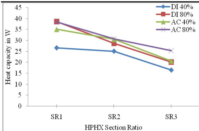
Figure 7: Effect of section ratio and filling ratio of different working fluids on heat capacity
