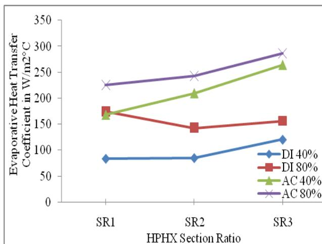
Figure 10: Effect of section ratio and filling ratio of different working fluids on evaporative heat transfer coefficient
