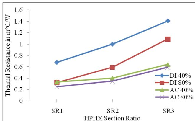
Figure 8: Effect of section ratio and filling ratio of different working fluids on thermal resistance
