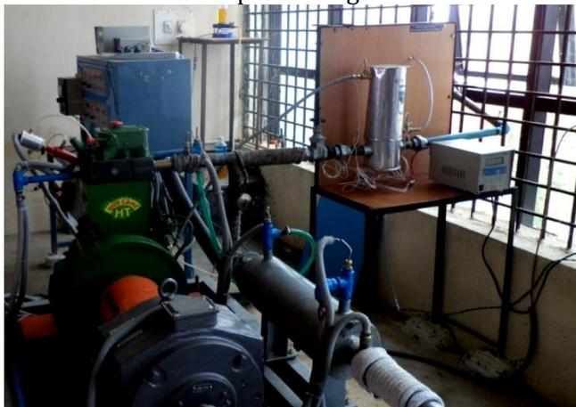
Figure 5: Installed and instrumented HPHX
