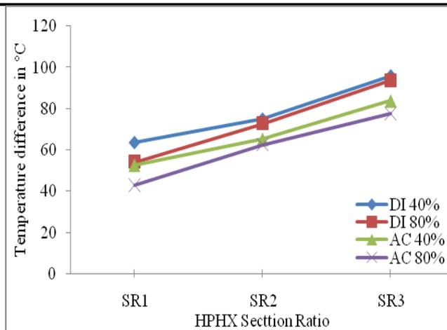
Figure 9: Effect of section ratio and filling ratio of different working fluids on temperature difference
