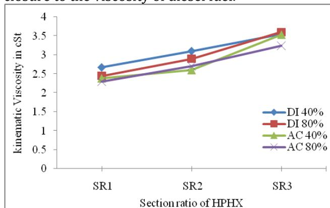
Figure 12: Effect of section ratio and filling ratio of different working fluids on kinematic viscosity of biodiesel
