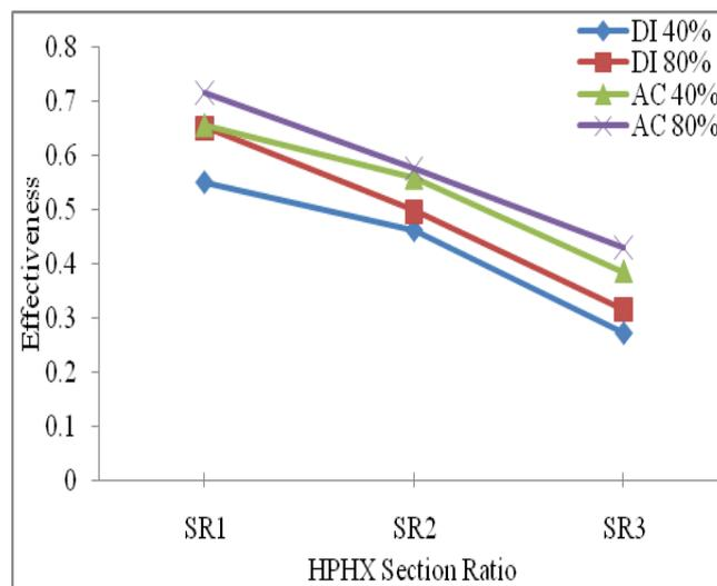
Figure 6: Effect of section ratio and filling ratio of different working fluids on effectiveness
