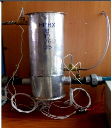
Figure 4: The Heat pipe heat exchanger assembly
