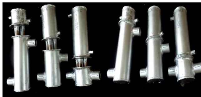
Figure 3: The HPHX assemblies before the thermal insulation and aluminum cladding
