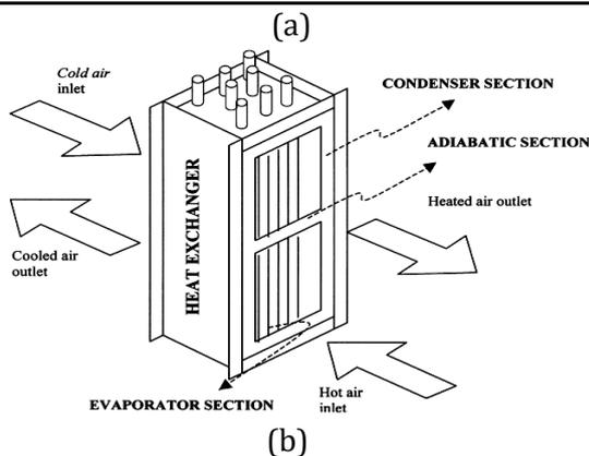
Figure 1: Typical Heat pipe (a) and the heat pipe heat exchanger (b).
