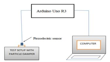
Fig 2: Proposed Schematic Experimental Test Set Up
