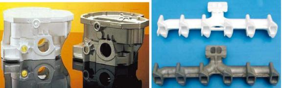
Fig 5: Trunk body casting and Foam pattern Fig.6 Exhaust manifold
