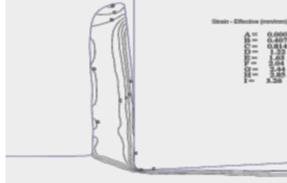
Figure 4.2. Plastic strain distribution
