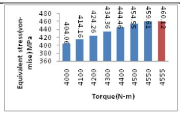
Figure 11: Equivalent stress in the universal joint at respective torque values
