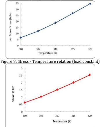
Figure 9: Strain-Temperature relation (load constant)
