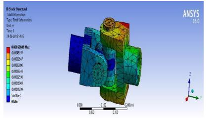
Figure 10: Total Deformation
