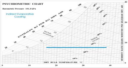
Figure 2 Psychometric Chart of Indirect Evaporative Cooler [5]
