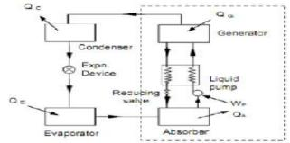
Fig.2. vapour absorption cycle
