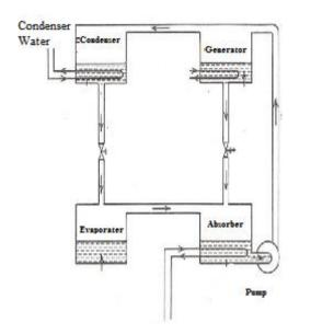
Fig. 3 Block diagram of VARS.
