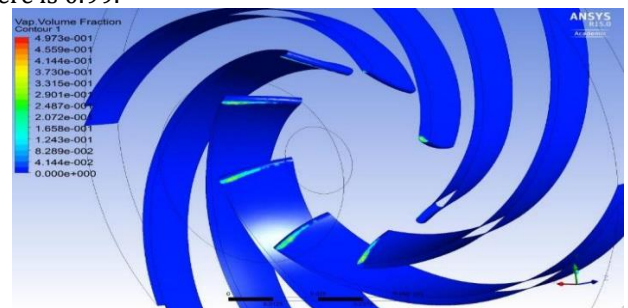
Fig. 5.2 Maximum vapor volume fraction on blades for Q/Q_D = 1.16
