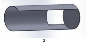
This component is made up of mild steel and it is used when cans are put in a rectangular box after which it holds the cans and main important factor is to grip it and get it crushed one by one. To design this component mild steel is taken on which design is marked then it is cut by hack saw machine according to the marked then this pipe structure is faced from both the ends. Gas cutting is done on the rectangular pipe using gas cutter. Then welding is done on the rectangular face.
