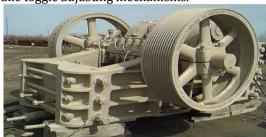
Figure-3 Jaw crusher
