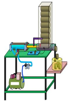
Fig. 1 Design of can crusher machine
