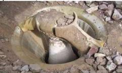
Fig. 4 Gyratory crusher
