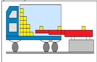
Fig.2 Working system of Telescopic Conveyor
