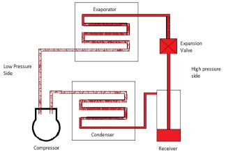
Fig. 3 Block diagram of VCRS.
