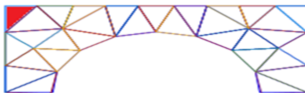
Figure 2: triangular grid generation in bridge
