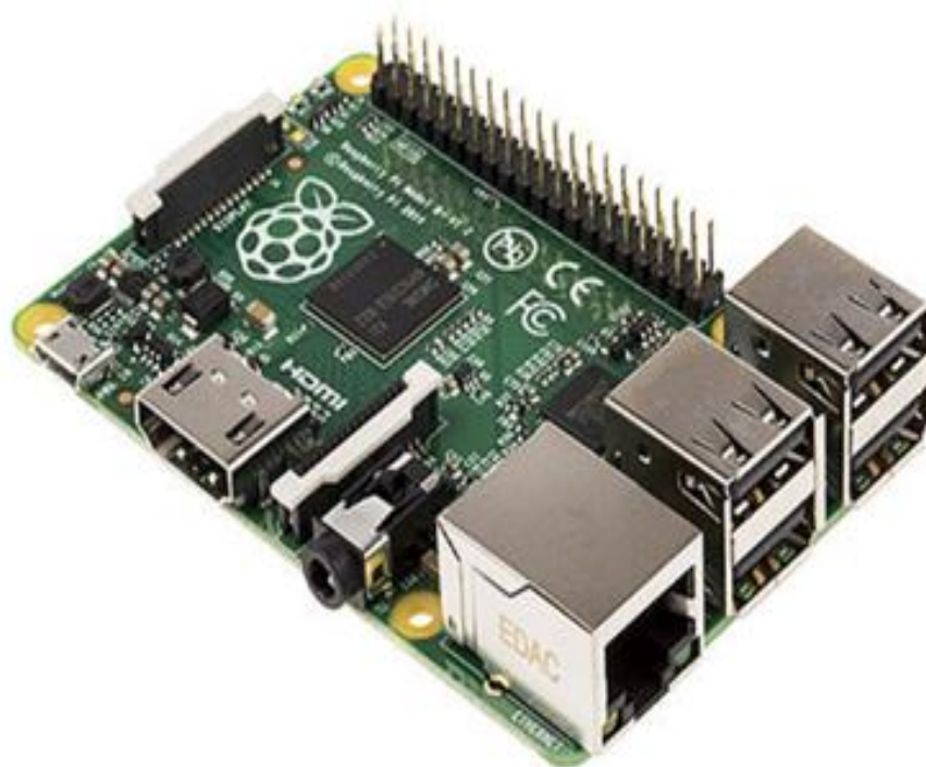
Fig 1. Implementation using Raspberry Pi kit
