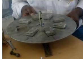
Fig.13. Placing Rotor on shaft
