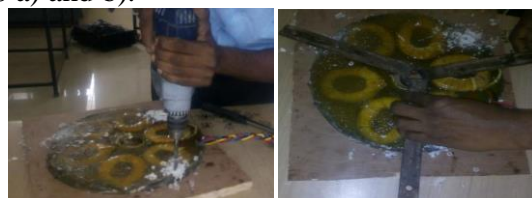
Fig 16 a) Drilling of casted stator
