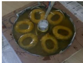
Fig.15. Stator coils casted in epoxy resin
