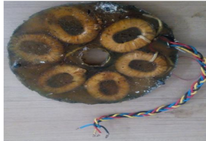
Fig.3.Stator cast in epoxy resin
