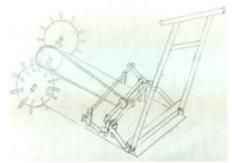
Fig 2 Isometric View of Rice Planting Machine
