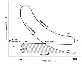
Fig. 6 PV diagram for EEVC
