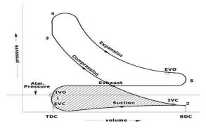
Fig. 4 PV diagram for LIVO
