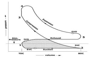
Fig. 7 PV diagram for LEVC
