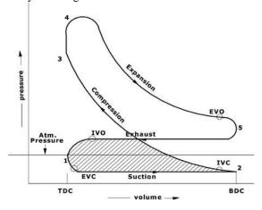
Fig. 5 PV diagram for EIVO
