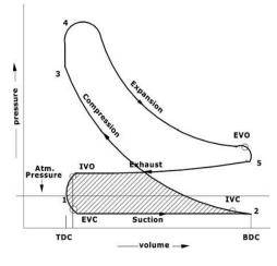
Fig. 9 PV diagram for LEVO
