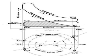
Fig. 1 Valve timing diagram in relation with PV diagram for conventional four-stroke engine.
