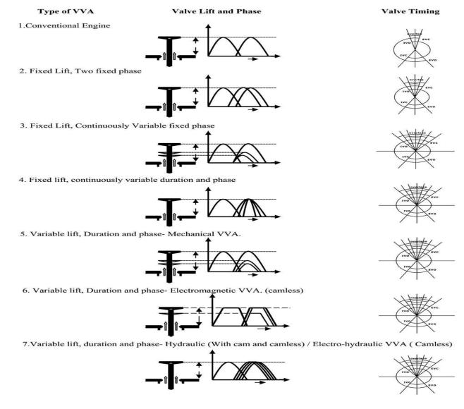
Fig. 10 Valve lift and Valve timing for various VVT mechanism
