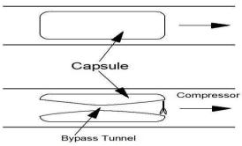
at the rear end of the capsule. If capsule cover too much area of the tube then, the air is not flow around the capsule and ultimately the entire column of air in the tube is being pushed ahead of the capsule and because of this there is friction between the air and tube walls is increases tremendously. Therefore to avoid this problem the compressor is fitted at the front of the capsule through which the air is flow which will not flow around the capsule and send it to bypass nozzle.
