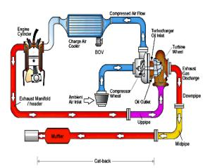
Figure: Process of Turbocharging
