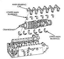
Fig.1 Assembly of Engine Bearing II.
