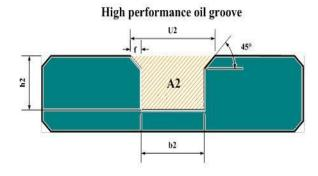
Fig.6 High Performance Oil Groove
