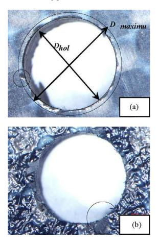
Figure: (a) Entry Delamination (b) Exit Delamination
