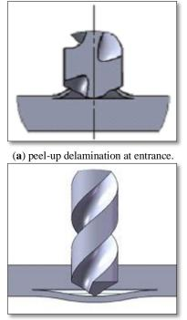
(**b**) push-down delamination at exit.
