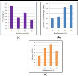
Figure 3. (a) Variation of density with reinforcement (b) Variation of tensile strength with reinforcement (c) Variation of hardness with 4.4.
