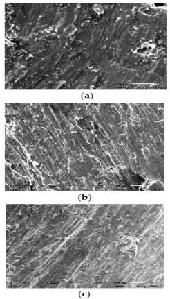
Figure 2. (a) Scanning electron microscopy (SEM) micrograph of specimen A (b) SEM micrograph of specimen B (c) SEM micrograph of specimen
