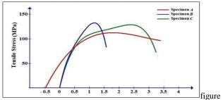
1. Stress-strain curve for specimens A, B, andC
