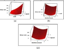
Figure 4. (a) Variation of wear rate with speed and load; (b) Variation of wear rate with load and reinforcement; (c) Variation of wear rate with speed and reinforcement.
