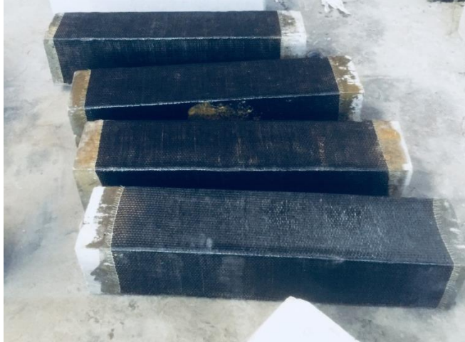
Beam after U-wrapping with BFRP fabric for flexural strengthening
