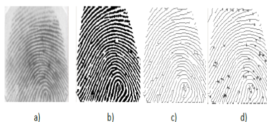
Fig. 11: Result of minutiae extraction with median filter pre-processing. a) original image; b) after binarization; c) after thinning; d) minutiae point extracted.
