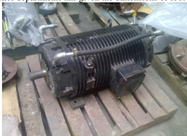
Figure 1:Foot mounting B3 type motor
